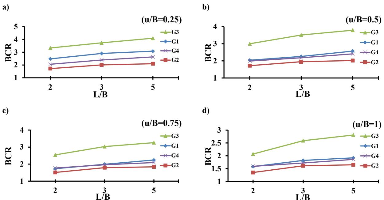
The corresponding trends in terms of BCR are summarised in Figure 10, which presents the BCR for G1 as a function of  $u/B$  for different reinforcement widths  $L/B = 2, 3$  and  $5$ . For any given  $u/B$ , BCR increases with  $L/B$ , confirming that wider reinforcement provides a larger confinement zone and engages a greater volume of soil. At
