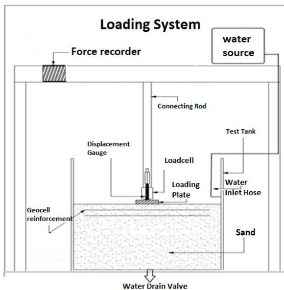
The vertical load transmitted to the footing was measured using a load cell connected between the jack and the model footing. The footing settlement was monitored by a dial gauge or linear displacement transducer mounted vertically on top of the footing plate. The data acquisition system used to record the applied load shown in figure 6.
