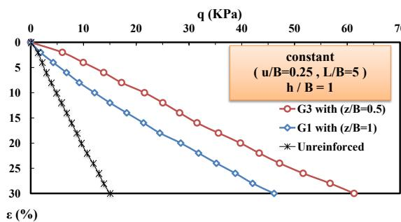
For each reinforcement width, both geocell types improve the footing response relative to the unreinforced sand, but the curves for G3 (smaller aperture) lie consistently to the right of those for G1, showing that the smaller-aperture
